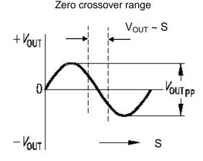
To convert small distance into a proportional electric signal, one can use a small soft iron part with definite width (e.g. b=1.8mm) to move over the face of the sensor. A linear signal up to 1.5mm can be obtained in this way. The sinusoidal signal gives a voltage output proportional to the distance in the zero crossover range.
