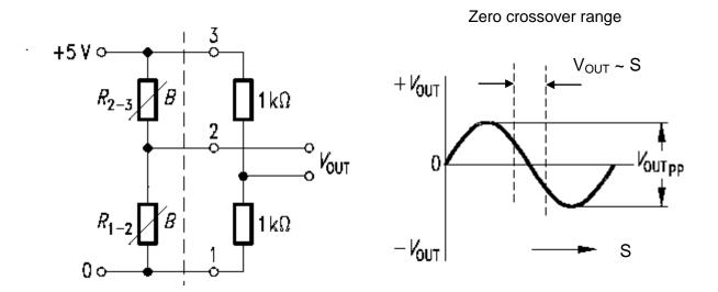
To convert small distance into a proportional electric signal, one can use a small soft iron part with definite width (e.g. b=1.8mm) to move over the face of the sensor. A linear signal up to 1.5mm can be obtained in this way. The sinusoidal signal gives a voltage output proportional to the distance in the zero crossover range.
