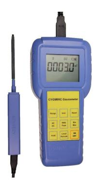
The Gaussmeter CYGM99C works according to Hall Effect measuring principle. It is a microcontroller-controlled instrument and can be used to measure DC/AC magnetic field strength of permanent magnet materials, motors, speakers, magnetic sensors/ transducers, other machines and instruments etc. with high resolution. It is powered with a rechargeable LiPo Battery (+3.7V) or via USB cable (+5VDC).
