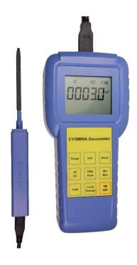
The Gaussmeter CYGM99A works according to Hall Effect measuring principle. It is a microprocessor controlled instrument and can be used to measure DC/AC magnetic field strength of permanent magnet materials, motors, speakers, magnetic sensors/ transducers, other machines and instruments etc. with high resolution. It is powered with 3 pieces of AA batteries (+1.5VDC) or via USB cable (+5VDC).
