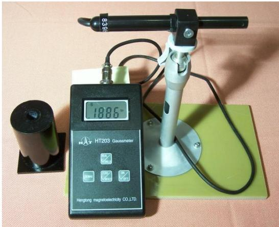
The Model CYHT203 is a hand-held Gauss-meter designed for accurate magnetic field measurements from 0.1mGs to 1.9999Gs. It can be used for measurements of very weak magnetic fields, for instance, earth magnetic field, environment and space magnetic fields, magnetic fields around shielded permanent materials and parts.
