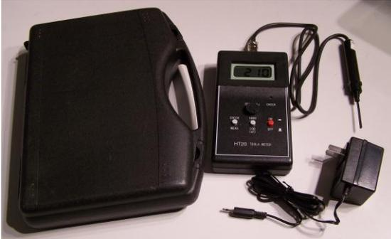
This Gaussmeter (Teslameter) is used to measure the magnetic field strength and to indicate the polarity of permanent magnets, DC coils and other DC magnetic fields.
