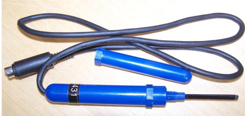
CYAP-D60B: axial probe  $\varnothing 6 \times 40\text{mm}$  (custom made)
