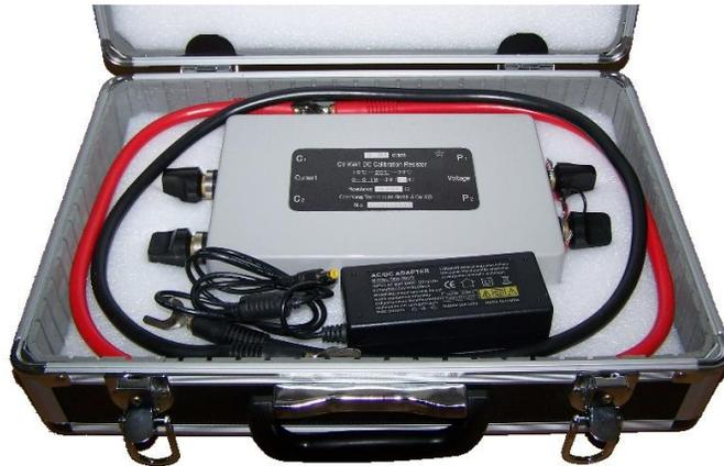
Before starting the measurement, the power supply +24VDC for the temperature control must be connected to the resistor, in order to control the working temperature of the resistor within the range 15°C ~ 30°C. The resistor needs to be preheated for 30~45 minutes before using it for measurement.
