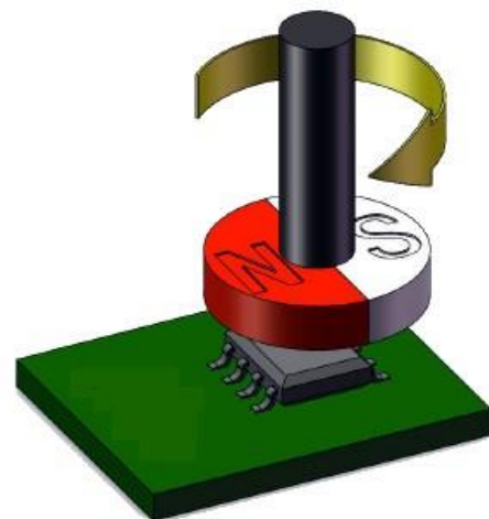
Installation schematic of CYAS-AM100 and magnet
