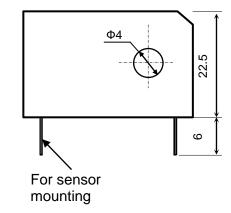
Dimensions: 31.5mm x 20.5mm x 22.5mm Aperture: Ø4mm
