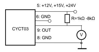
The value of the pull-up resistor R should be selected in order to get a current of 4-5mA flowing through the pull-up resistor. For instance the pull-up resistor is  $24V/4.5mA=5.3k\Omega$  if you use a power supply +24VDC.
