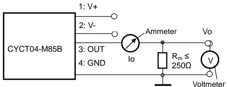
Relation between Input and Output (for  $R_m=250 \Omega$ ):
