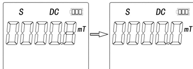
**Note:** You must reset the Gaussmeter before you start a new measurement after you have changed the measuring range (12) and AC/DC mode (11).
