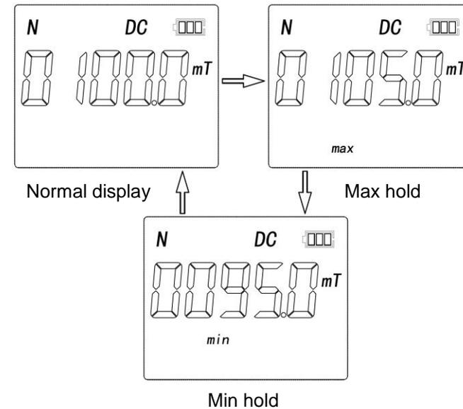
**Note:** Under the Max/Min mode the display changes only when the actual measuring value is larger/smaller than the last value displayed. Therefore you must firstly reset to the normal mode by using button (6), if you need to measure a magnetic field, which is smaller/larger than the previously measured value.
