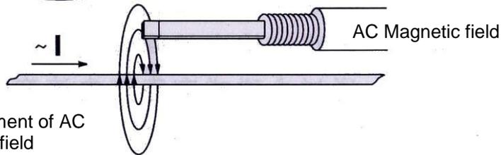
Measurement of AC magnetic field generated by AC current
