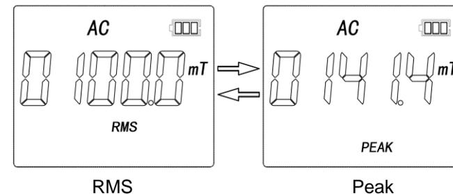
**Note:** AC measuring results are assumed as sinusoid magnetic field signal. The RMS or amplitude of fundamental wave is displayed on LCD.
