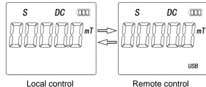
sets it to local control. Pressing the "Local Remote" button (7) on the instrument also changes the mode.
