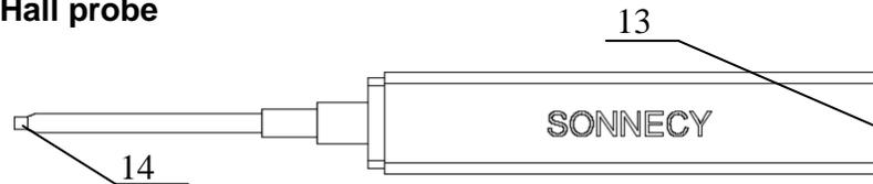
13: USB micro B port for measuring instrument
