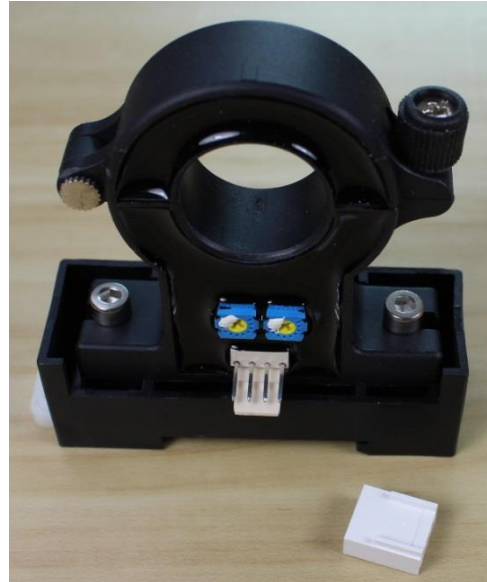
Sensor with Molex Connector (The distance between the bottom und the middle of hole is 54.8mm)
