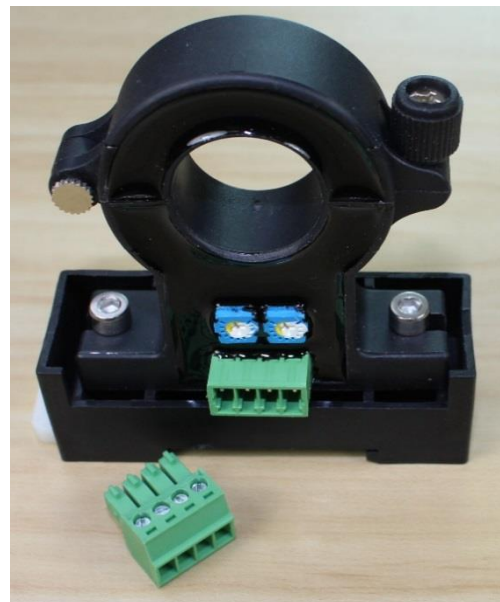
Sensor with Phoenix Connector (The distance between the bottom und the middle of hole is 54.8mm)
