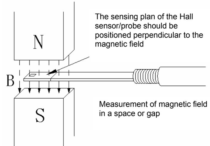
Put the concave side, i.e. the side with a small circle mark of the probe on the surface of the measured magnet or at the measuring point of a magnetic field carefully.
